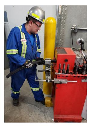
Before using the skiving machine ensure guides are out and lid is in place.
