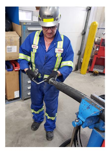
Manual skiving is performed when you are unable to safely keep the hose from turning in the skive machine. You can use manual skiving to remove small amounts of rubber that are left over from skiving with machine.
